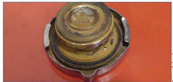
Figure 6: Radiator Cap (Pressure Cap): Weak springs, old rubber gaskets or a failed pressure test are signals for replacement. Caps have a limited lifetime and should be replaced when a new radiator is installed. A worn out pressure cap will not hold pressure as high as it should and will not open as per originally designed. A pressure cap not opening will cause severe damage, but a worn out pressure cap will cause constant additional stress on the radiator that will shorten its life expectancy.
