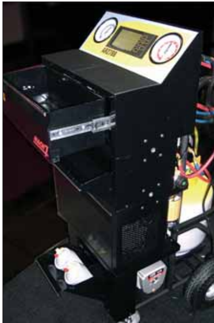
The GPS Products AR2788 a/c service machine has an all-metal body with three drawers in front and one at the bottom, for storing spare filters.
