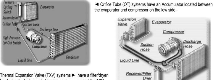
Thermal Expansion Valve (TXV) systems ► have a filter/dryer located in the high side between the condenser and the TXV.
